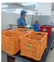
Figure 28: Measuring the specific gravity by potato gauge.
